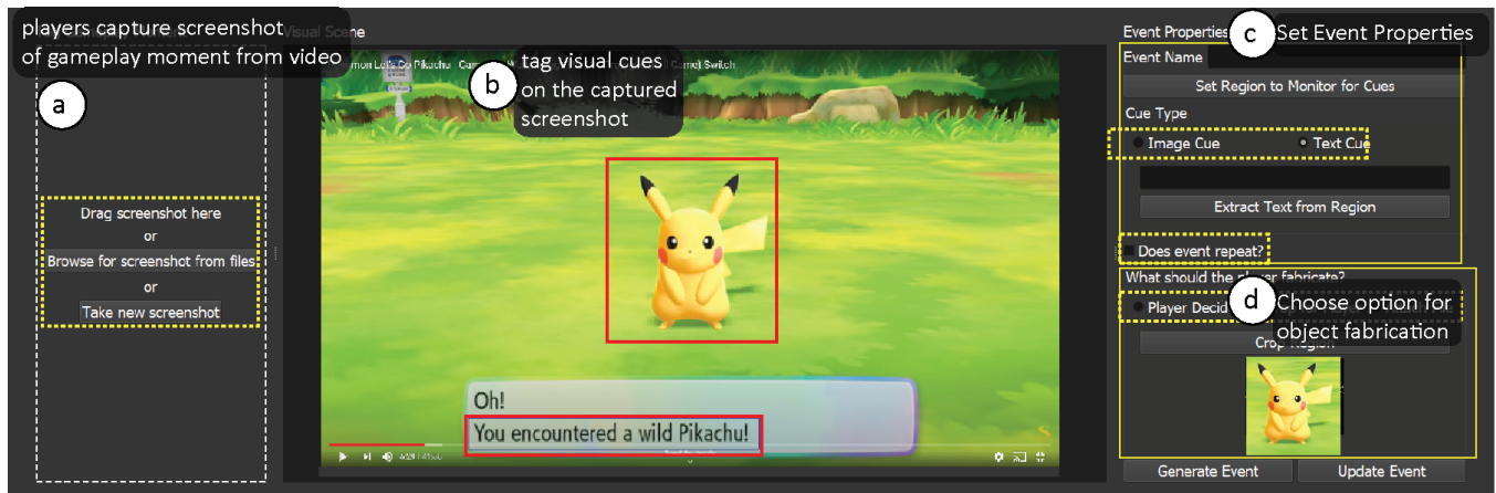
Figure 3: To integrate fabrication events, designers use FabO's designer interface to (a) capture the screenshot of the gameplay moment (b) tag the on-screen visual content as cues, such as text or images, (c) set event properties, and (d) choose option for object fabrication.
